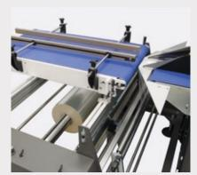
Loading belt to recognise and load the products with conveyors, palettes or cups or directly joined to the previous line.
