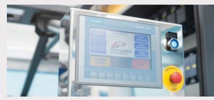
Intuitive touch screen for simple format change. The touch screen can rotate in 3 different Electric box on view, positioned up high, positions to allow the operator to work on all sides of the machine, front, back and side.
