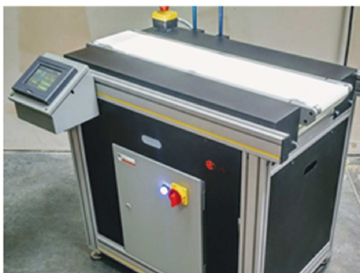
1m backlit conveying section
